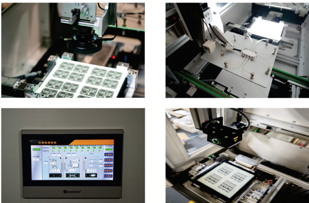
Figure 14. More device details of AOI system.
